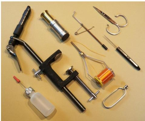
**Vise** - A simple, sturdy vise is the basic foundation for fly tying. There are many types, ranging widely in quality, features, and price. Most vises use simple, cam-actuated, adjustable steel jaws to firmly grip a wide range of hook sizes. Just make sure it's sturdy so it will last for many years.
