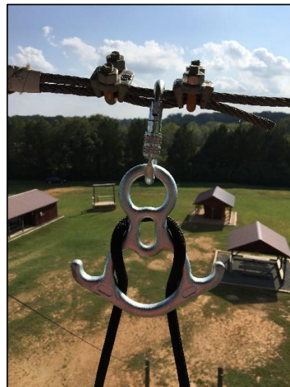
The rappel rope has been fed through the rescue 8 at the rope midpoint and the steel carabiner has been screwed closed.
