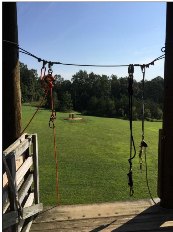
Complete rappel rigging at MSR including all tethers. Note the participant tether is just on the left leaning against the railing.
