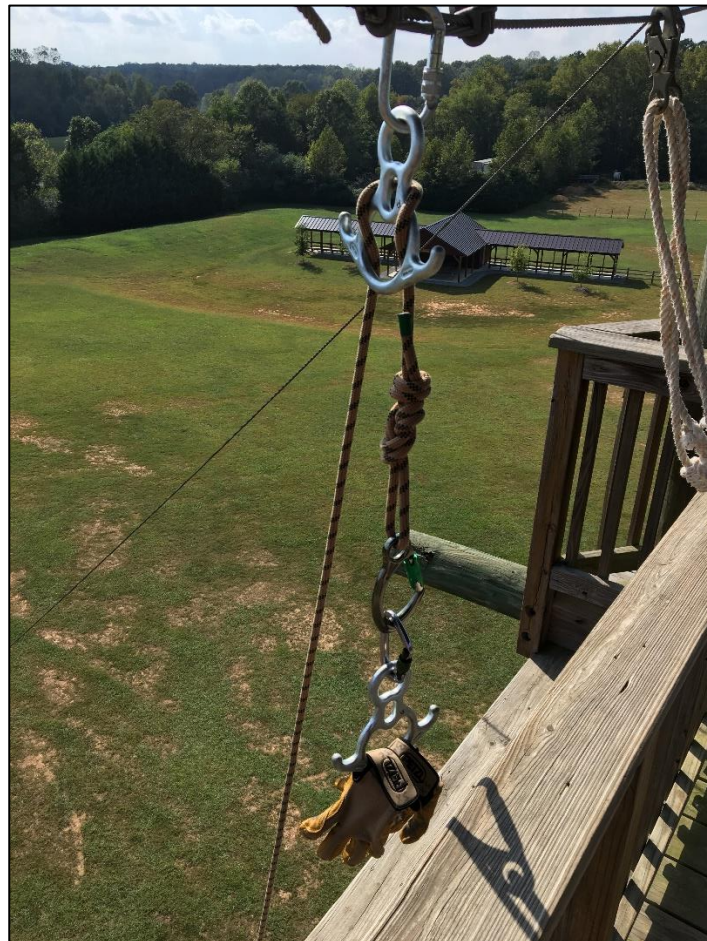
Belay rope tied with a figure 8 on a bite through a tri-act captive eye carabiner and fed through the rescue 8 belay device. Note the rescue 8, carabiner and rappel gloves are already in place.
