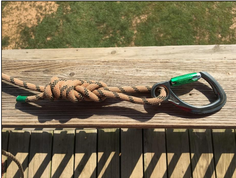
Captive eye carabiner tied with a figure 8 on a bite and properly backed up.
