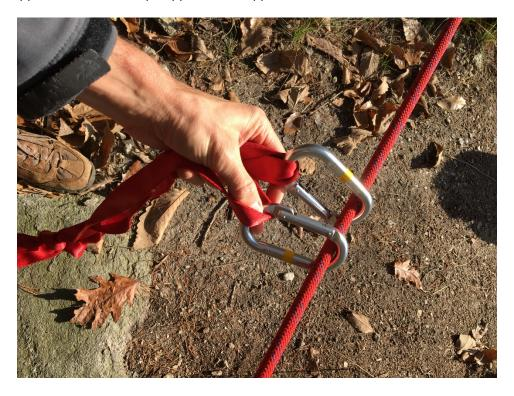
As the participant moves along the tether system one leg of the lobster claws can be removed and clipped around the obstacle (carabiner, tree, knot, etc.). Then the following carabiner can be clipped around the obstacle. One of the lobster claw legs must remain clipped to the tether system at all times. Participants must be instructed in proper use of the lobster claws and the tether system during the safety briefing at the start of the program day.
