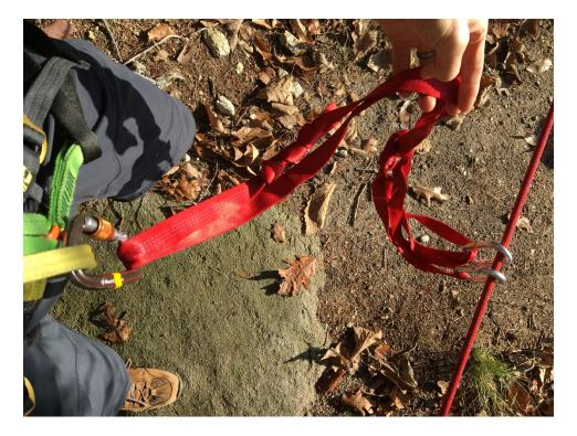
The two carabiners on the loops must be clipped to the rope of the tether system. The two carabiners should be clipped to the tether rope opposite and opposed.
