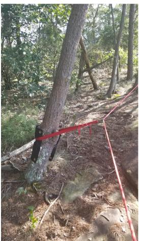
Place a canvas pad on the leaning pine tree with the growth. Place the tree guard over the growth, then basket hitch a 15' length of webbing, pull the rope toward the tree and attach it using a carabiner. With the webbing and canvas pad placed below the growth on the tree, the webbing will remain in position and not "walk" up the tree.
