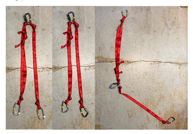
The locking carabiner will be clipped to the participant's harness when he/she reaches the start of the tether system. This should not be removed from the harness until the participant is on belay at the rappel station or has been transferred to an intermediate tether.
